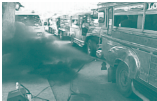
Particulate emissions, some of which exit the tailpipe as black smoke, increase significantly when vehicles are in poor state of repair or engines are improperly adjusted, such as this heavy-duty diesel-powered bus.
