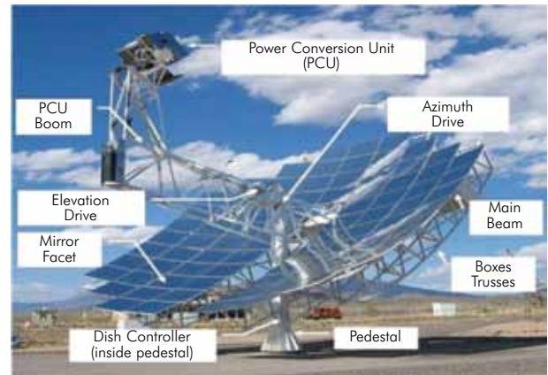
Figure A.10: Dish-Engine Photo with Major Component Identification
