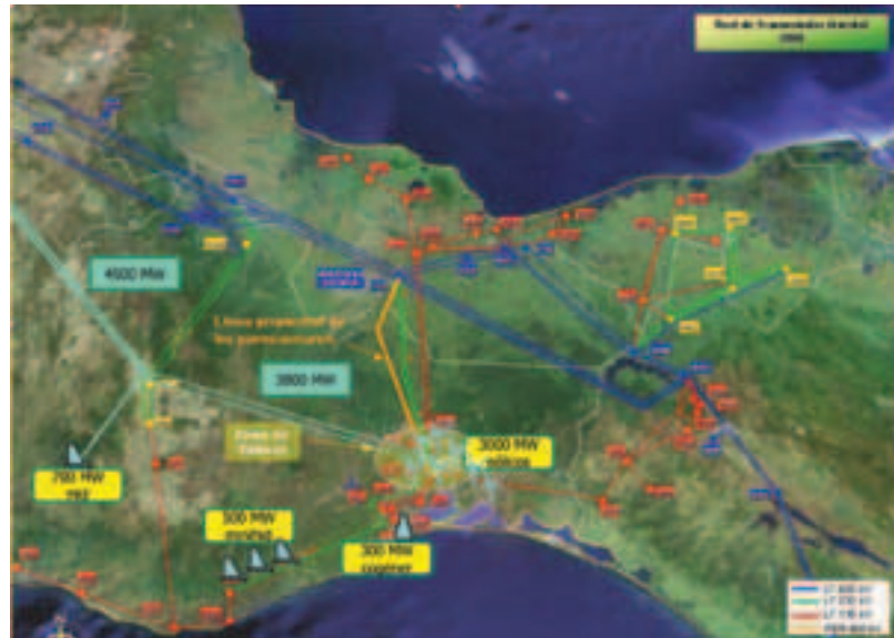
Figure A.10: Existing Transmission Network and New Transmission Needs in La Ventosa Region
