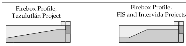
Figure 4.5 Firebox Differences Between Stoves
