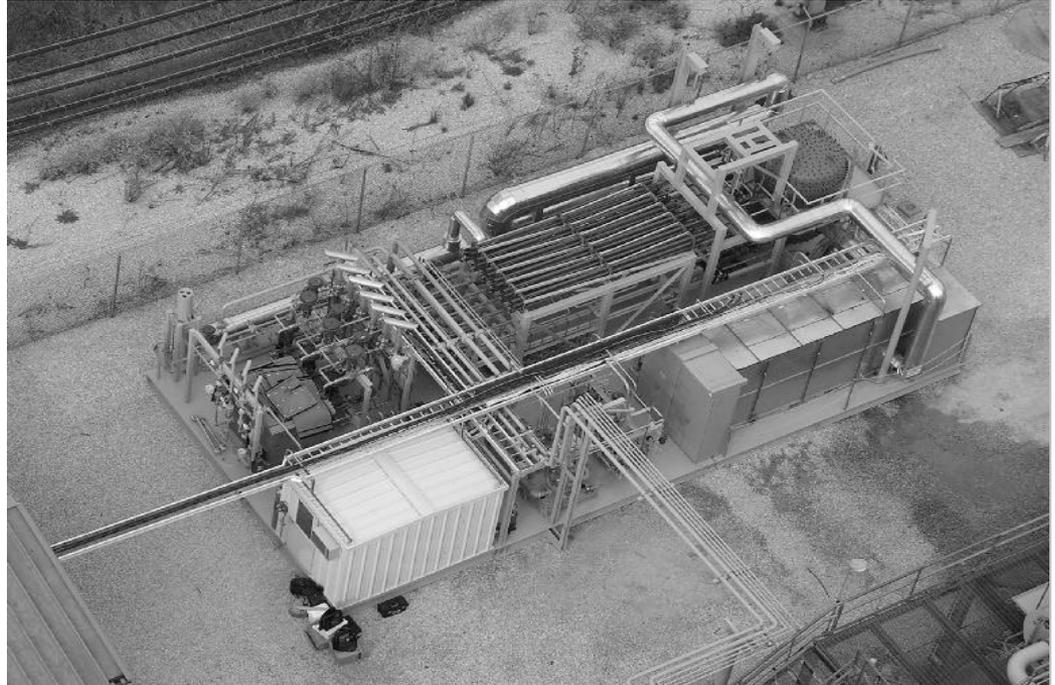
Subscale engineering prototype ITM test unit at APCI's Sparrows Point gas plant
