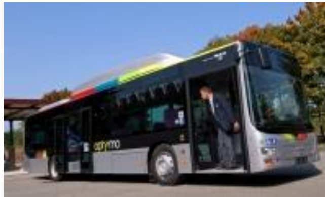
Figure 2: LPG bus; tanks are located on the roof
