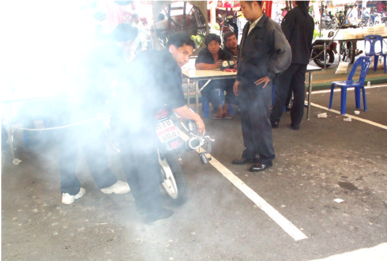
Figure A3.7 Measuring the White Smoke Level
