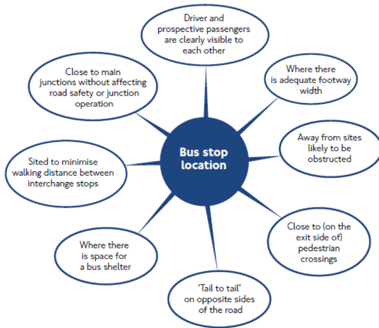
Figure H2: Considerations for Bus Stop Locations (14)
