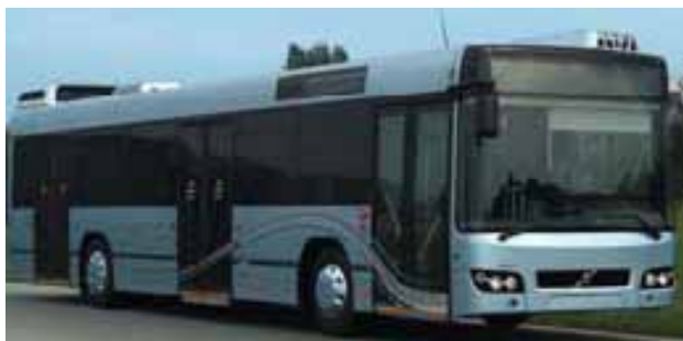
Example - Volvo 7700 Citybus – 32 passenger seats but capacity for up to 95 passengers with low floor access and standing - 9L Volvo Diesel, 12m option
