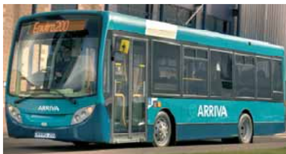
Example – Alexander Dennis Enviro 200 – from 8.9m to 11.3m with between 24 and 40 seats with low floor access
