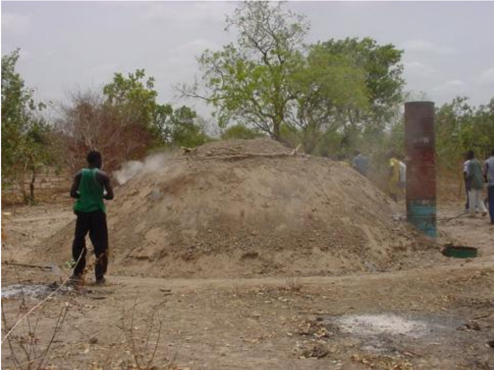
Photo 12: Improved charcoal production with the Casamance kiln –Senegal
