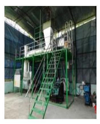
Biomass based gasifier 20 – 30kWP
